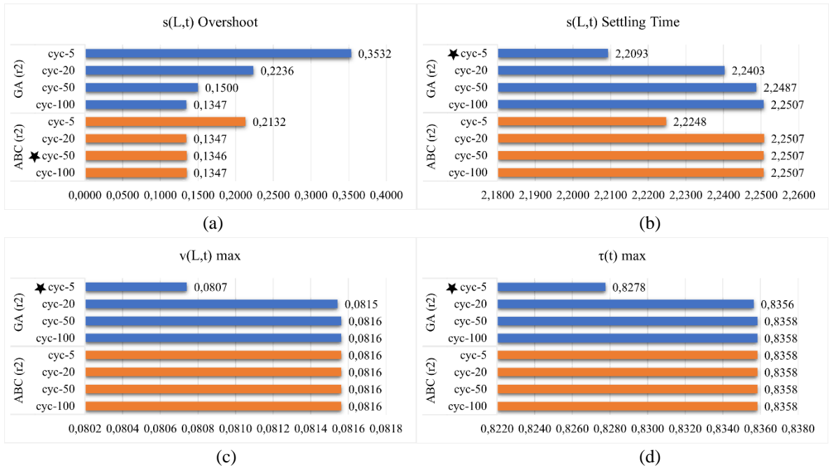
Fig. 3. Performance comparisons for r_2 optimization, (a) s(L, t) overshoot, (b) s(L, t) settling time, (c) maximum end point oscillation, (d) maximum torque value
