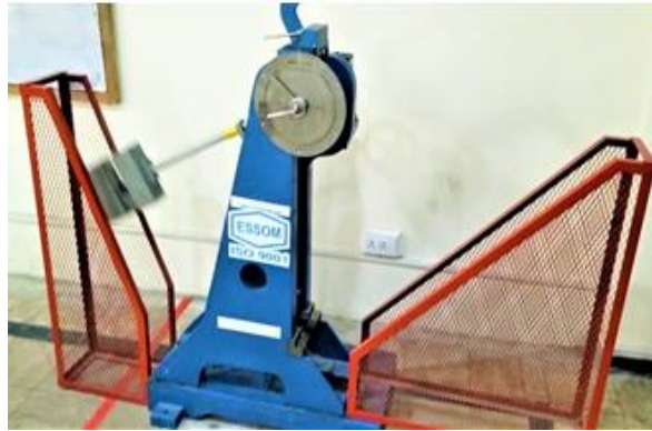
Fig 2. Experimental set up (Impact Testing)
