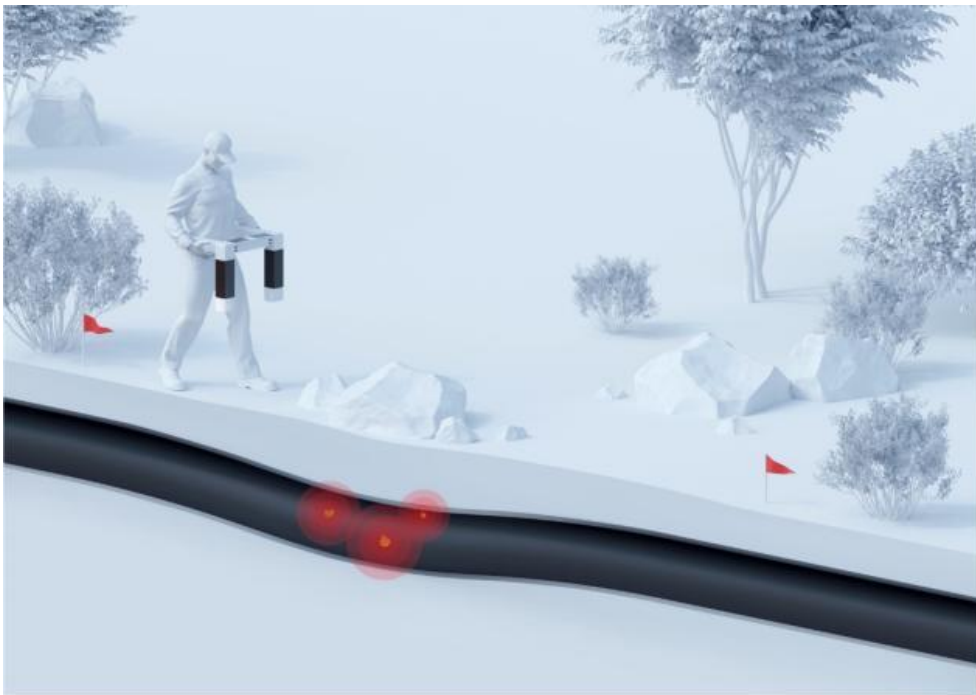
Fig. 2. A simple schematic of the MTM-G method showing localized magnetic dipoles caused due to stress (red dots) which are then detected by the aboveground equipment.
