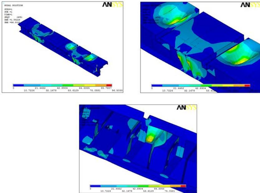
**Fig. 16.** Van Mises Compound Stress Results of the fixed part hinge
