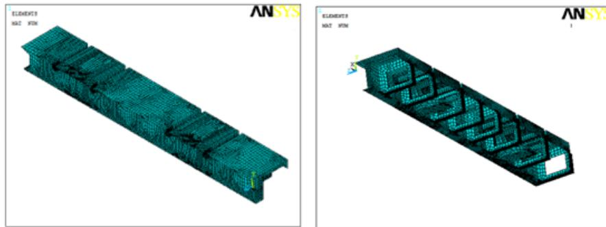
**Fig. 11.** Mesh representation of the fixed part hinge
