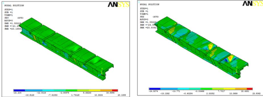
Fig. 18. Deflection Value Results of the fixed part hinge
