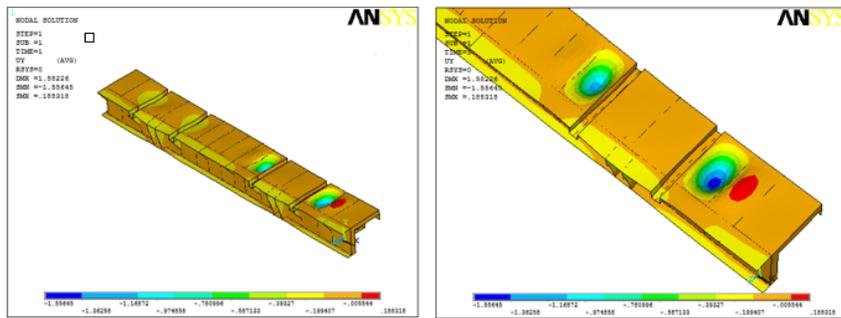
**Fig. 17.** Shear Stress Results of the fixed part hinge
