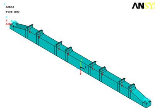
Fig. 6. View of beam compressive loads
