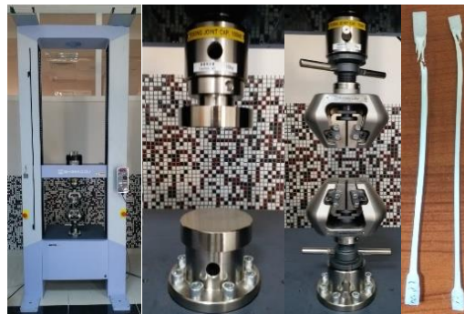
Fig. 4. Shimadzu AGS-X 100 kN universal testing machine [12]
