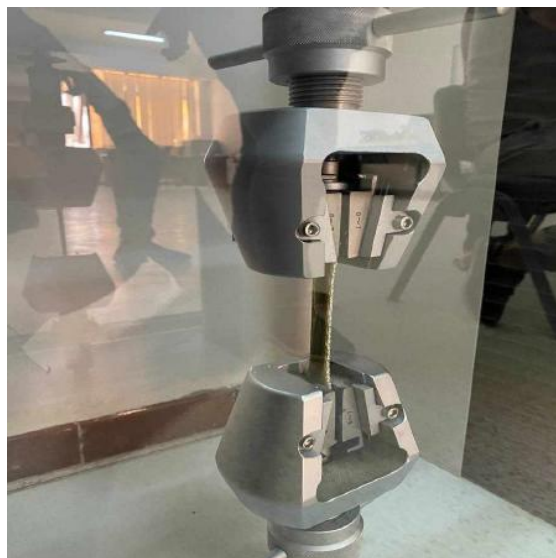
Fig. 5. Tensile test of a composite specimen
