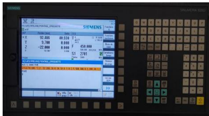
Fig. 9. Programming with the G-code
