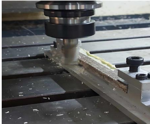
Fig. 12. Execution of the specimen machining program
