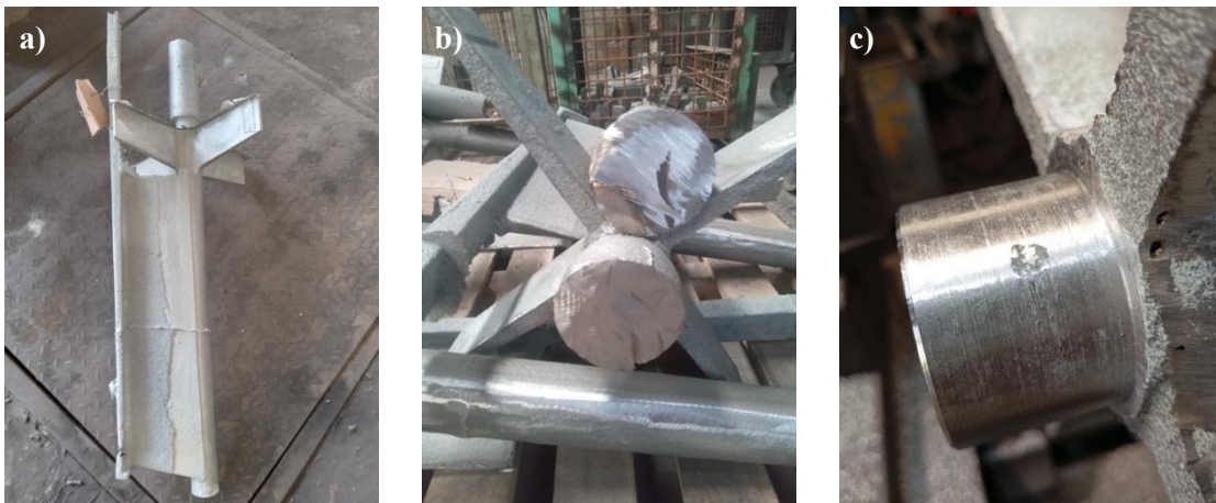
Fig. 13. Casting trial specimen 1 produced at an actual pouring temperature of 1591 °C: (a) as-cast component exhibiting uniform surface finish and minimal metal-mold interaction defects; (b) pre-machining condition after riser removal; and (c) partially machined section revealing a shallow peripheral shrinkage porosity associated with localized feeding deficiency during final solidification.
