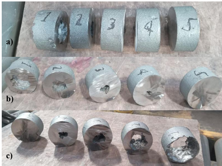
Fig. 18. Sectioned evaluation of the feeder of casting trial specimen 4 (actual pouring temperature: 1564°C; 1 – top section, 5 – feeder-shaft-interfacing section): (a) external surfaces of the sectioned samples showing overall surface integrity; (b) upper cross-sections revealing extensive interdendritic shrinkage cavities and centrally concentrated feeding-related porosity; and (c) lower cross-sections showing partial soundness in distal regions, particularly to the section closest to the shaft.
