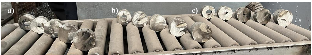
Fig. 17. Sectioned evaluation of the feeders of the fan shaft specimen cast at (a) 1578°C [specimen 2, target: 1580°C], (b) 1578°C [specimen 3, target: 1570°C], and (c) 1591°C [specimen 1, target: 1590°C]. Specimen 2 and specimen 3 show similar feeder utilization despite having different results, considering both specimens were cast at the same pouring temperature.
