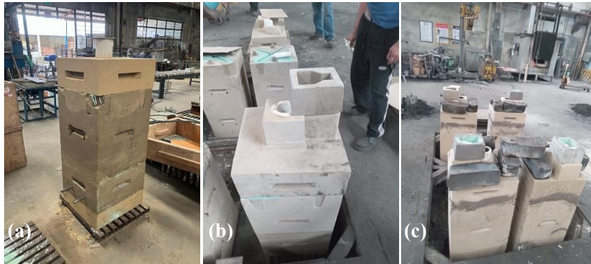
Fig. 7. Final mold assemblies for casting trials: (a) closed mold assembly highlighting the structural interfaces between shaft body, blade junction and feeder neck; (b) pouring cup with sprue extension positioned to support gravity filling and exothermic sleeve fitted; and (c) mold fitted with counterweight for stability during pouring.
