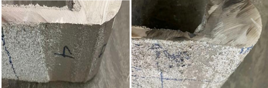
Fig. 12. Specimen from trial cast batch 1 showing surface quality degradation along the shaft length. Section taken from the middle of the shaft (left) and the end of the shaft (right).
