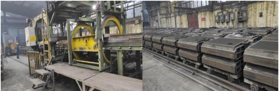
**Fig. 1.** HWS SINTO HSP-3 horizontal molding line [30]
